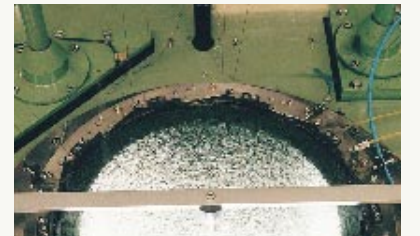
Each size and garment part is knitted to shape on various knitting machines with needle beds of different diameters. This gives the garment a good shape and fit and exceptional comfort.
